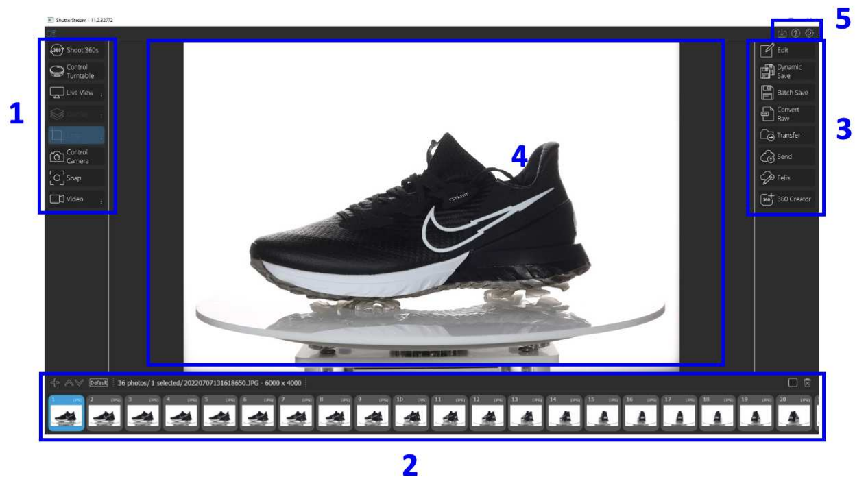
Figure 2.1: Visere Captura overview:(1) Image Composition and Capture Tools, (2) Image Viewing and Thumbnail Gallery, (3) Image Processing and Output Tools, (4) Live View and Image Viewing Window, and (5) Import, Help, and Settings.
